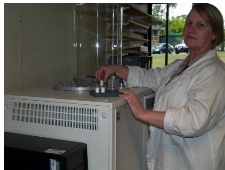
Leco carbon analyser measures C by combustion process
